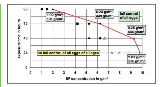
Fig. 8. Exposure time and concentration of sulfuryl fluoride to obtain full control of eggs of *P. interpunctella* at 27°C; bold symbols directly taken from Tab. 1; data for other symbols by nonlinear regression; square: 1 day old eggs, triangle: 2 day old eggs, circle: 3 day old eggs; diamond: 4 day old eggs; lines indicate necessary conditions for full control of eggs of all ages: Multiplication of exposure time and the indicated figures results in the ctp<sub>100</sub> for these conditions.
